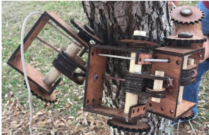
Figure 8. Prototype Testing Shows Pivot points between Modules are the same for both Clamping and Helical Generation
