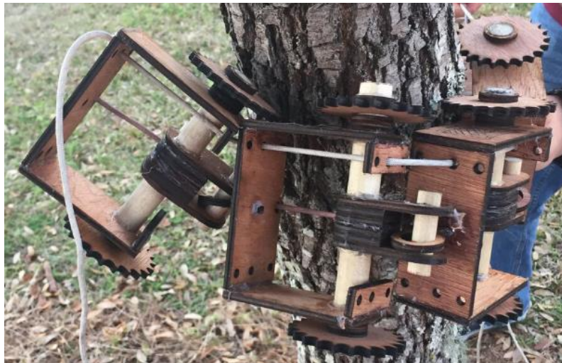
Figure 7. Version 9 – Pivot points designed into the module connectors
