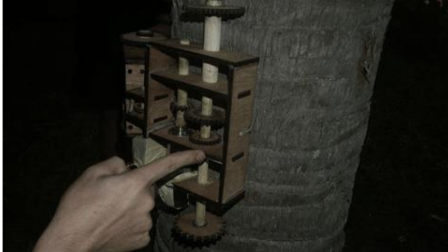
Figure 10. Verification of Helix Generation Coupled with Clamping and Motion
