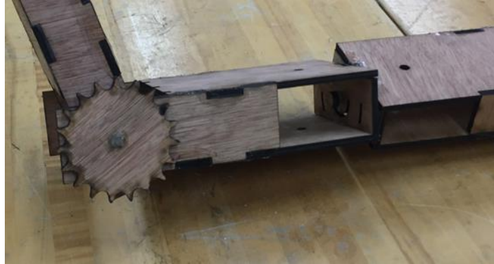
Figure 4. Version 5 - It includes a third DOF for rotation between modules
